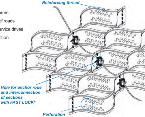
**VERTICAL LOADS REDISTRIBUTION** - load redistributes onto the neighboring cells, reducing stress on the underlying basement and creating the "flexible slab" effect
