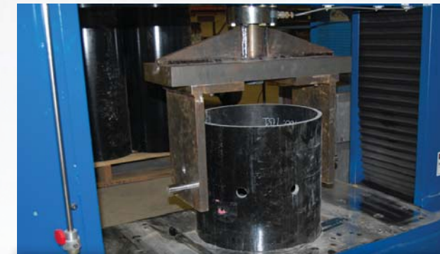
Bolted Connection Test - Parallel
