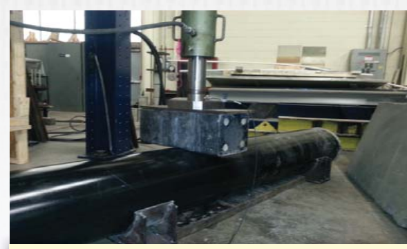
Crush Test on Concrete Filled Pile
