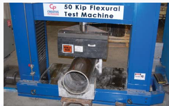
SUPERPILE Crush Strength Test Set Up
